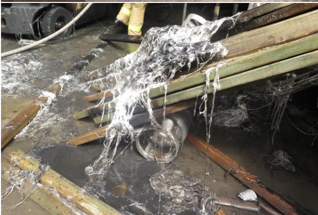
Fire initially involved scaffolding containment mesh, formed of high-density polyurethane and fiberglass reinforced banding. The burning mesh separated and fell igniting fresh fires on lower levels and at ground level, adjacent to the basement. Fire intensity of the burning mesh was severe, resulting in fire entry into the basement and explosion of multiple stored gas cylinders within the basement.
