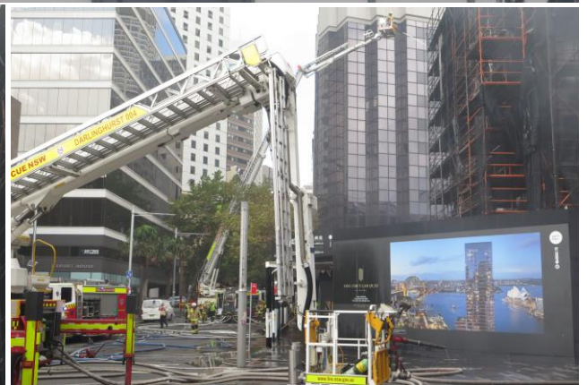
Ladder Platform 1 established cutoff of fire burning the perimeter scaffold mesh on the Bravo side. The aerial master stream was also used to cool the steel tower supporting the tower crane.
