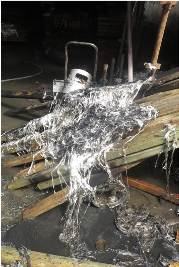
Fire initially involved scaffold containment mesh, formed of high-density polyurethane and fibreglass reinforced banding. The burning mesh separated and fell igniting fresh fires on lower levels and at ground level, adjacent to the basement. Fire intensity of the burning mesh was severe, resulting in fire entry into the basement and explosion of multiple stored gas cylinders within the basement.
