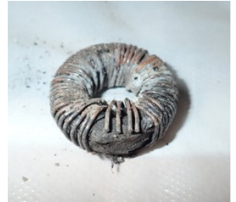
Figure 5 (right) the damaged toroid transformer
