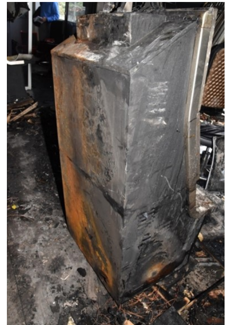
Figure 2 (right) Photo showing the left side of machine 4. Note no oxidation on this side, and the inverted "V" pattern of oxidation on the rear of the machine.
