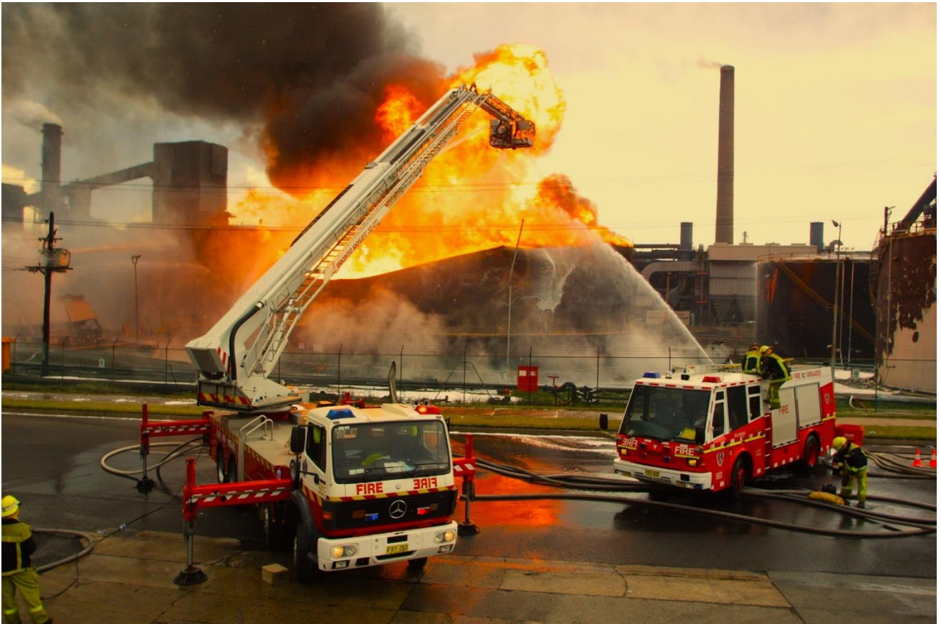
Upper: Pumper 49 supplies water to Ladder Platform 503. Lower: Ladder Platform 503 and Super Pumper 503 direct cooling streams onto the wall of the burning ethanol tank.
