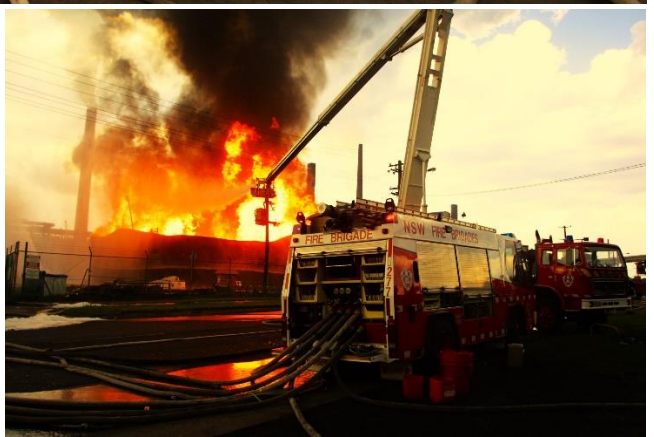
From Division A Firefighters operate multiple master streams, protecting heavily threatened Tank 14 and cooling the steel wall of the burning ethanol tank.
