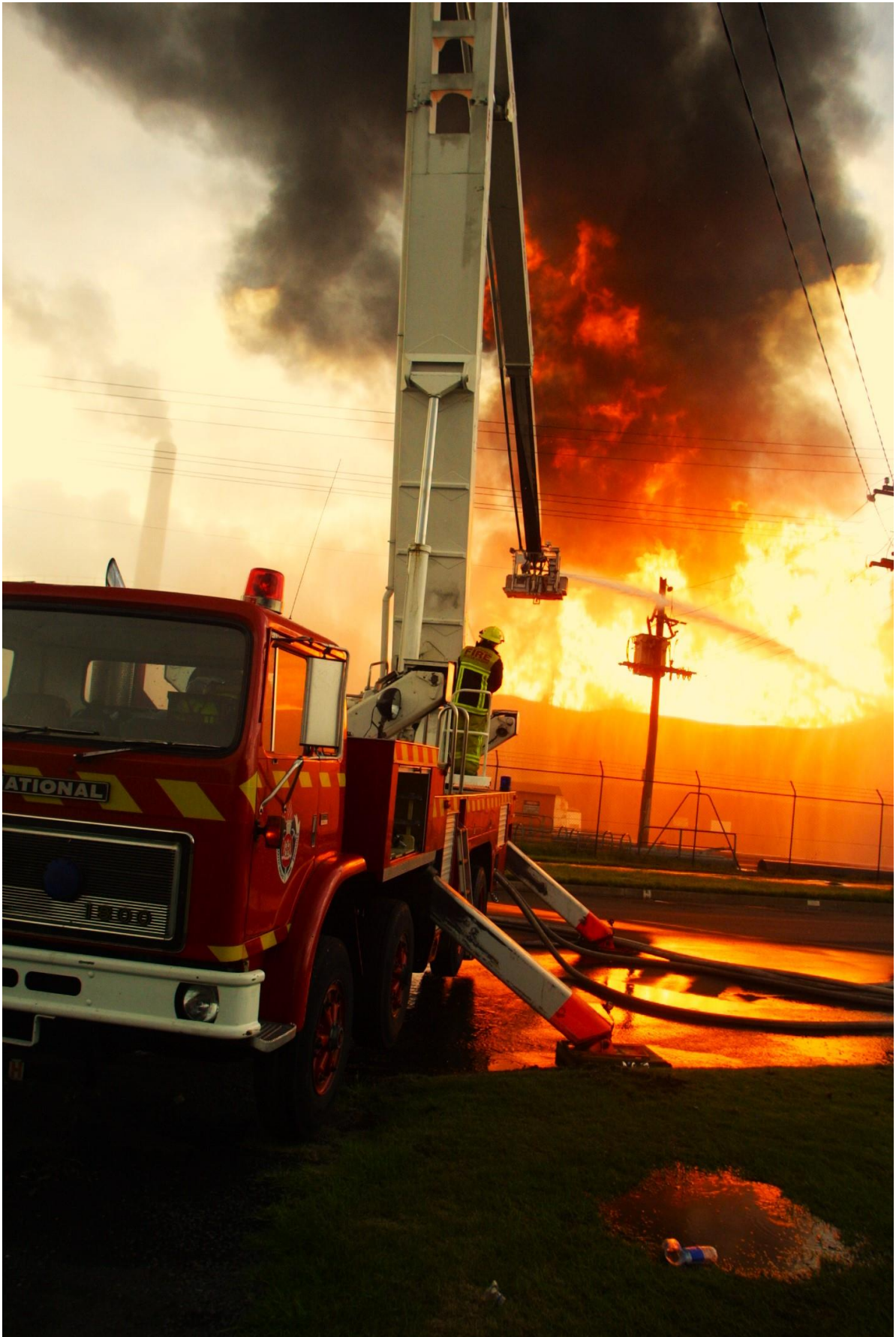
Hydraulic Platform 21 operated by Senior Firefighters Dave Phillips and Jeff Wilson alternated the aerial stream between Tank 14 and the wall of the burning ethanol tank.
