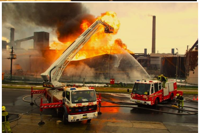
Upper and Middle: As the incident progressed additional protection streams were placed in operation, securing exposure tanks under threat. Lower: Ladder Platform 503 and Super Pumper 503 alternate master streams Between the burning tank wall and exposure tanks.
