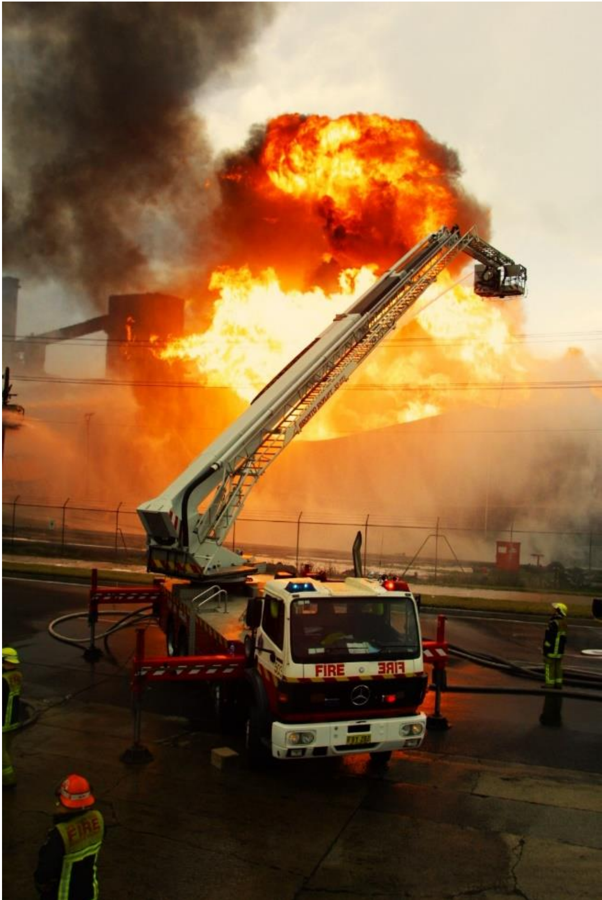
Ladder Platform 503 firefighters direct the aerial master stream onto the wall of the involved ethanol tank, protecting the integrity of the steel wall of the tank. These operations assisted to prevent tank failure.
