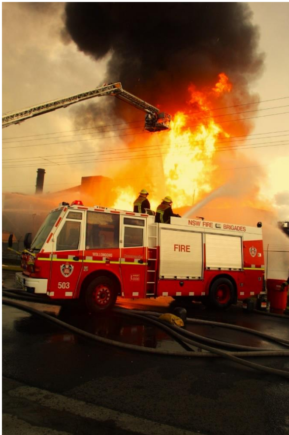
Upper left: 210 Station firefighters direct a protective stream onto the cage of Hydraulic Platform 21 and a pole mounted electricity transformer. Ladder Platform 503 and Super Pumper 503 direct large diameter cooling streams onto the sides of the involved tank and Tank 8.
