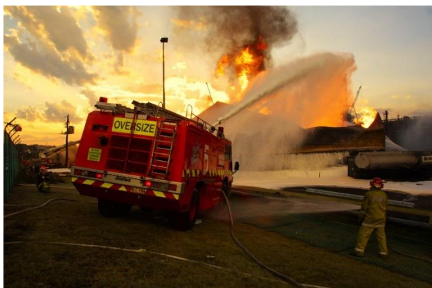
Aviation Rescue and Fire Fighting (ARFF) firefighters commence to attack the fire with the appliance monitor foam stream, delivering 7,000 litres of finished foam solution onto the fire at a rate of 3,600 litres per minute. Just as the foam attack was commencing strong winds impacted the fireground, greatly intensifying fire conditions. Note fire activity on the right side of the tank in the middle photograph. These flames were impacting Tank 14. The ARFF crews provided extremely professional support to operations.
