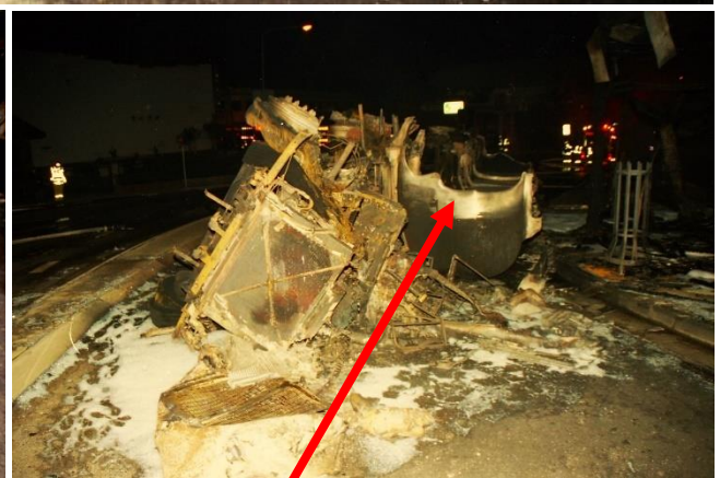
Severe fire damage to the tanker. The aluminium tanker shell “melted down” as the fire burnt lower. The remnants of the tanker shell (shown by arrows) are indicative of the levels of flammable liquid at the time of extinguishment. When attacking a flammable liquid fire, the objective of firefighters is to get foam onto the surface of the flammable liquid.
