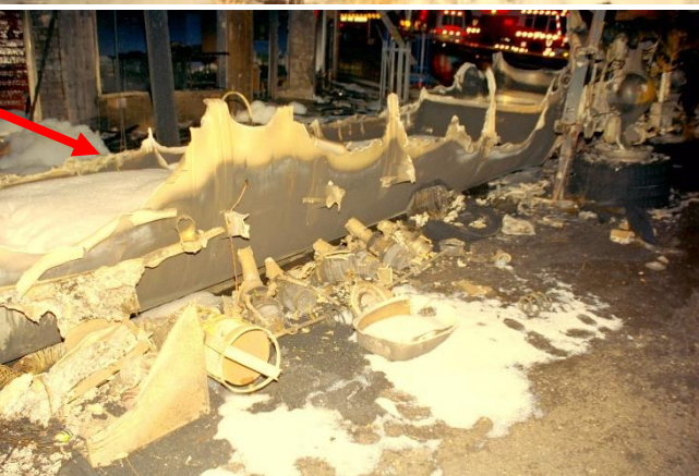
Severe fire damage to the tanker. The aluminium tanker shell “melted down” as the fire burnt lower. The remnants of the tanker shell (shown by arrows) are indicative of the levels of flammable liquid at the time of extinguishment. When attacking a flammable liquid fire, the objective of firefighters is to get foam onto the surface of the flammable liquid.
